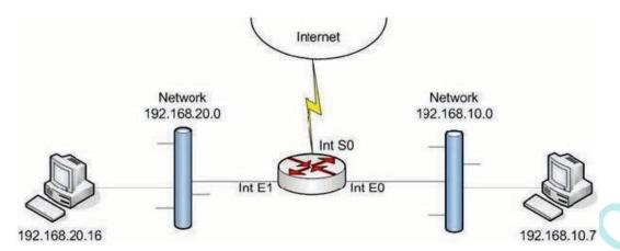
The objective is to allow two hosts, 192.168.20.16 and 192.168.10.7 access to the Internet while all other hosts are to be denied Internet access. All hosts on network 192.168.10.0 and 192.168.20.0 must be allowed to access resources on both internal networks. From the following, select all the access list statements that are required to make this possible.
