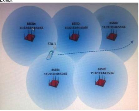
ABC Company has deployed single channel architecture (SCA) solution to help overcome some of the common problems with the client roaming. The figure shows the overlapping coverage area of multiple APs in ABC's network. In this network all APs are configured with the same channel and BSSID. PEAPv0/EAP-MSCHAPv2 is only supported authentication mechanism.
