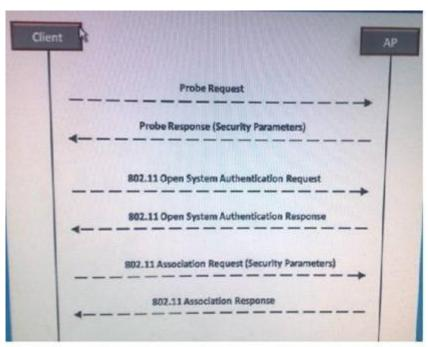
The illustration shows the 802.11 association procedure from the IEEE 802.11 standard. In a WPA2-Enterprise network what process immediately flows the 802.11 association procedure?
