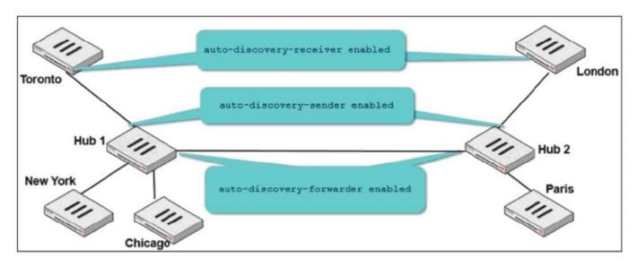
Two hub-and-spoke groups are connected through a site-to-site IPsec VPN between Hub 1 and Hub 2. The administrator configured ADVPN on both hub-and-spoke groups.
