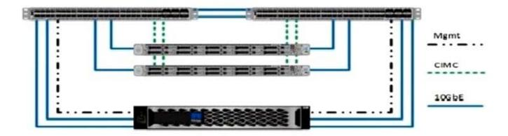
You have designed a FlexPod Express solution that uses a NetApp ONTAP controller, Cisco UCS C-Series servers, and Cisco Nexus 3000 Series switches, as shown in the exhibit.
