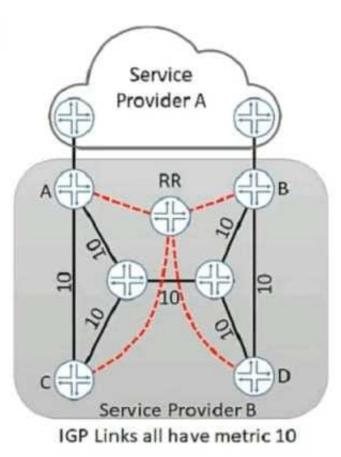
You work for service provider B that wants to implement a hot potato routing policy on the network so that router C uses link C-A to reach service provider A\\'s advertised routes and router D uses link D- B to reach Service Provider A\\'s advertised routes C uses the network on router B. Referring to the exhibit, what are two design actions that would satisfy the requirements? (Choose two.)
