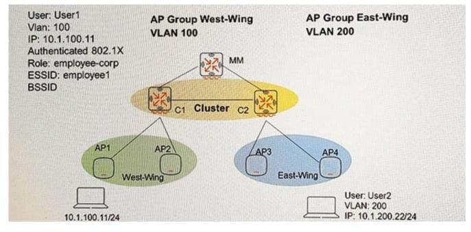
Controllers are configured in a cluster as shown in the exhibit. These are the network details.
