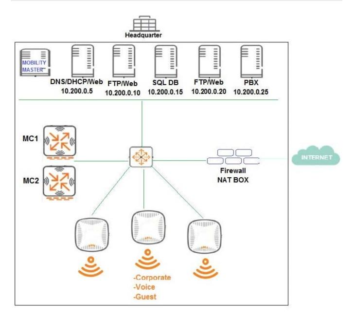
An organization provides WiFi access through a corporate SSID with an Aruba Mobility Master (MM)Mobility Controller (MC) network that includes PEF functions. The organization wants to have a single firewall policy configured and applied to the employee role.
