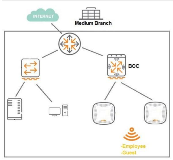
A 7008 Branch Office Controller (BOC) is deployed in a remote office behind a core router. This core router does not support 802.1q encapsulation. The Mobility Controller (MC) is the gateway for two tunneling mode SSIDs, as shown in the exhibit.
