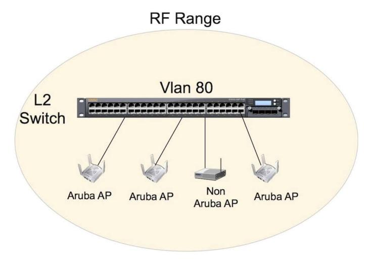
Referring to the diagram provided for this question, an employee brought an unauthorized AP from home and attached the LAN port to the cubicle Ethernet port. All Aruba APs and AMs as well as the employee AP are in VLAN 80 and within RF range of each other. No traffic from the wired or wireless network has passed through the unauthorized AP yet, but the AP began wireless broadcasts.
