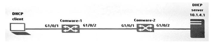
The physical interfaces for Comware-1 and Comware-2 switches in the exhibit are configured in routed mode and OSPF. Both switches have the three subnets in their routing tables. The administrator wants to use DHCP to assign addressing information to the users. Based on the exhibit, where should the administrator configure DHCP relay?
