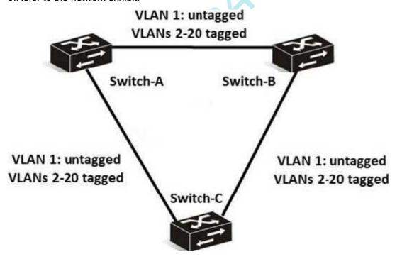
A network administrator has created a layer 2 network based on the design shown in the exhibit. Switch-A and Switch-B are distribution layer switches. Switch-C is an access layer switch.
