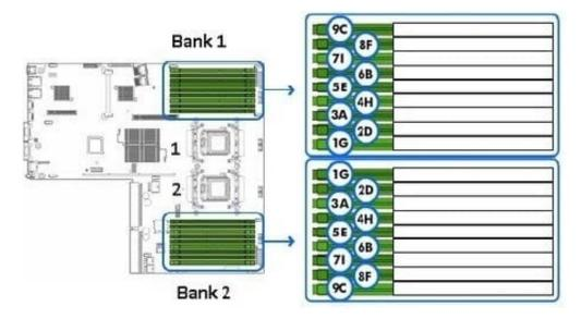
A. Four quad-ranked LRDIMMs are supported across all memory channels. The server balances capacity automatically.
