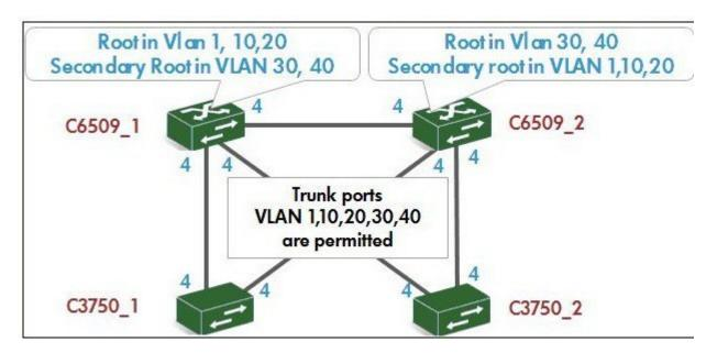
The Cisco network of an Example Corp, shown in exhibit is configured with PVST+. What will happen if you change Spanning Tree mode to MST on C3750\_1?
