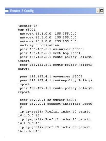
Network 16.2.0.0 /16 is advertised by Router 1 and Router 2 into BGP. All traffic from AS-65002 destined to 16.2.0.0 /16 enters AS 65001 via the Serial 3 interface of Router 1. The administrator prefers that this traffic enter AS 65001 via interface Serial 4 of Router 2. Which configuration change is most likely to achieve the desired results?
