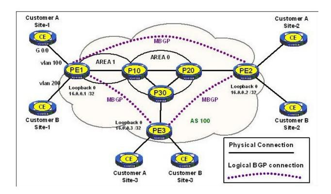
A provider of MPLS services configures MPLS Layer-3 VPN services for two customers. Each customer has three branch offices that will be interconnected by MPLS Layer-3 VPNs. The address blocks chosen by the customers for each site are shown in the following chart:
