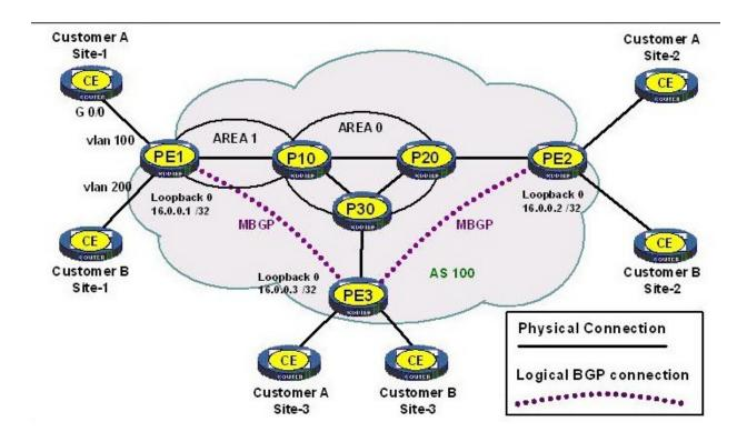
A provider of MPLS services configures MPLS Layer-3 VPN services for two customers. Each customer has three branch offices that will be interconnected by MPLS Layer-3 VPNs. The following are address blocks chosen by the customers for each site as shown in the chart:
