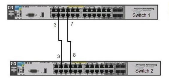
VLAN1: Ports 1,3,5,8-24 (untagged) VLAN 10: Ports 2,4,6,7 (tagged)
