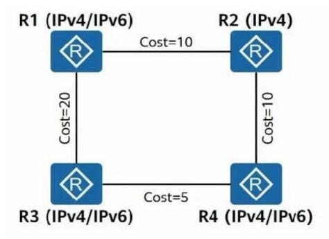
A. If you want IPv4 and IPv6 network computation to form the same shortest path tree, you need to run the ipv6 enable topology ipv6 command to enable the IPv6 capability in the IS- IS process.
