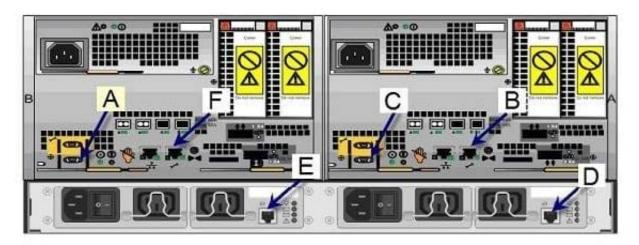
Which letter indicates the location of the port where the SPS sense cable would be installed on SP A?
