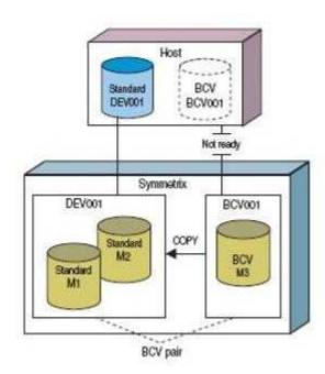
Based on the exhibit, how is data copied during the restore operation from a TimeFinder/Mirror BCV device (M3) to a mirrored standard device (M1 and M2)?
