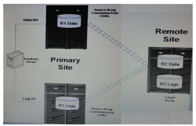
A database server has its logs stored on a volume on the log source Symmetrix V-Max array and its data stored on a volume on the data source Symmetrix V-Max array. Both source Symmetrix V-Max array frames replicate data to the target Symmetrix V-Max array at the Remote site.
