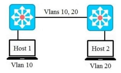
A network administrator needs to configure the switches to allow traffic to communicate from Host 1 to Host 2. Which recommended switch port mode should the interconnecting switch ports be configured?
