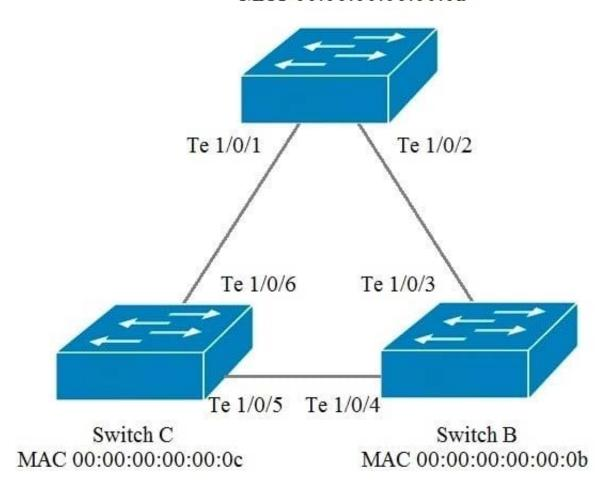
The exhibit represents a topology with all Dell EMC N4000 Series switches with RSTP enabled. In addition, the switches are using the default configuration on all ports and protocols. Which port number will be blocked by spanning tree?
