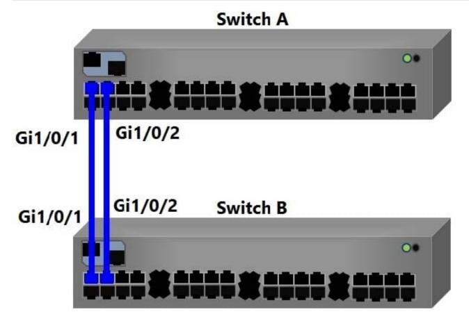
Switch A and Switch B are connected to each other. Both switches use interfaces Gi1/0/1 and Gi1/0/2. Switch A has a Spanning Tree priority of 8192 and Switch B has the default priority. Which interface becomes the root port?
