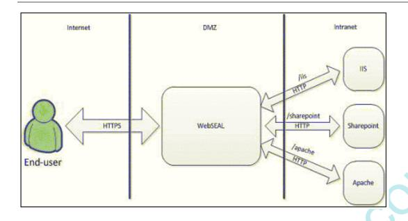
The exhibit displays a high-level setup of a basic Security Access Implementation. All communication between end-user and WebSEAL happens over HTTPS. The communication between DMZ and Intranet is HTTP-based. What information is gathered if 'pdweb.https' is enabled on WebSEAL?
