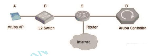
the wireless user's laptop is associated with an Aruba AP's Virtual AP profile in tunnel forwarding mode.
