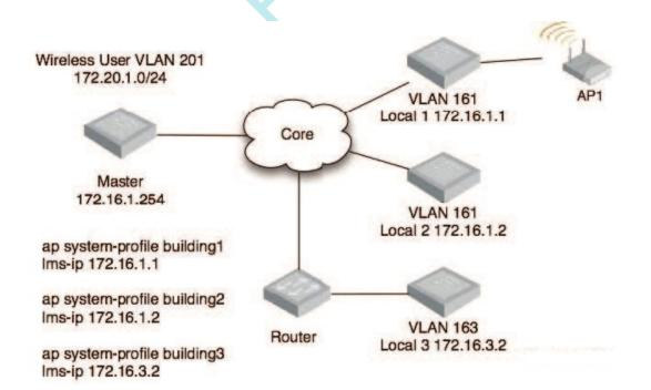
All controllers are configured with the wireless user VLAN 201. A wireless user associates with AP 1. Only L2 mobility is enabled.
