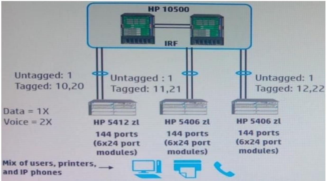
The network architect is planning network addresses for the VLANs shown. The company is using the private 10.0.0.0/8 space. Which guidelines should the network architect follow?
