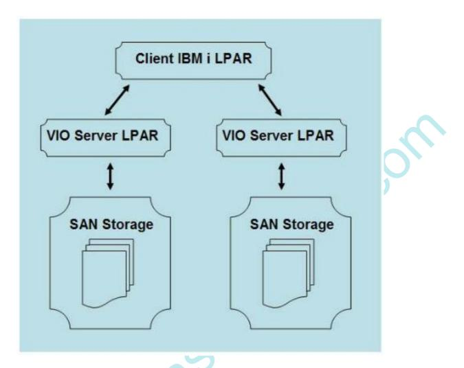
Considering both the host and client partitions, what is the minimum number of vSCSI adapters required to support this disk configuration?
