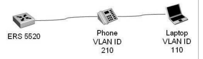
The following steps were performed to successfully configure the Ethernet Routing Switch (ERS) 5520 to
