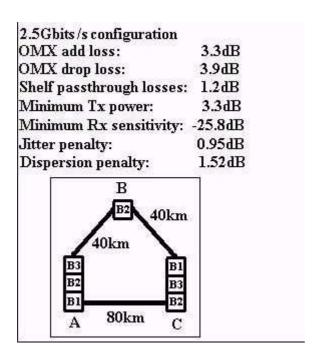
A. 28.87 dB; (There is no need for an amplifier because the un-amplified optical link budget is not exceeded.)
