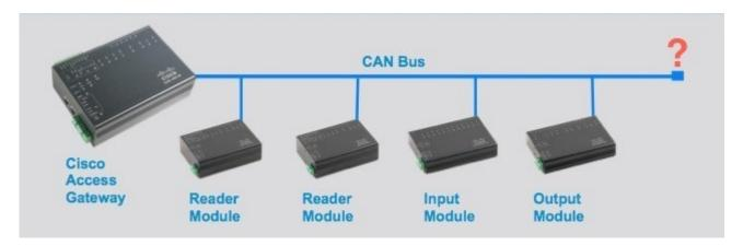
One or more expansion modules is connected to the Cisco Access Gateway via a CAN bus. How should the CAN bus wires be connected after the last module in the chain?
