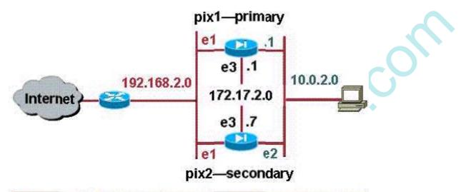
pix2(config)# failover lan interface LANFAIL ethernet3 pix2(config)# failover lan unit secondary pix2(config)# failover lan key 1234567 pix2(config)# failover lan enable pix2(config)# failover
