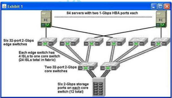
You are designing a new SAN. The existing SAN uses eight 32-port 2-Gbps Fibre Channel switches. Two of the switches are deployed as core switches, and the remaining six switches are deployed as edge
