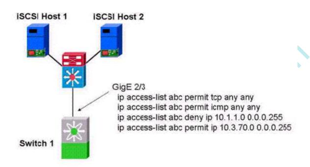
A.The traffic is allowed to pass through the interface because there is an implicit permit applied.
