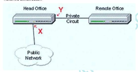
A customer has two sites, each with an IP Office linked via a private digital line (E1/T1). The head office is connected to the public network through a digital exchange line. The remote site gains access to the public network via the head office.
