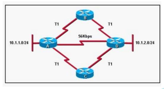
A. If EIGRP is the routing protocol, the equal cost paths ABD and ACD will be installed in the routing table by default.
