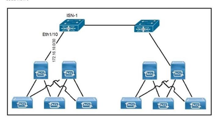
Refer to the exhibit. A customer implements Cisco ACI Multi-Site with default MTU settings between two sites. Which configuration should be applied on the interface Eth1/10 on the ISN-1 device?
