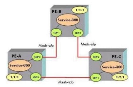
A new router named PE-D is to be directly connected to PE-C and is required to be added to the existing VPLS 300. The design requires the least amount of signaling, the least amount of configuration changes for existing sites and the new site has to have access to all existing sites.
