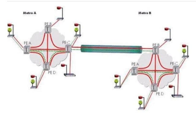
Assuming there is a full mesh of mesh-SDPs between the PEs within each metro network and a spoke-SDP between PE-C of Metro A and PE-B of Metro B. how is traffic forwarded from PE-A in Metro A to PED of Metro B? Select the most accurate statement.
