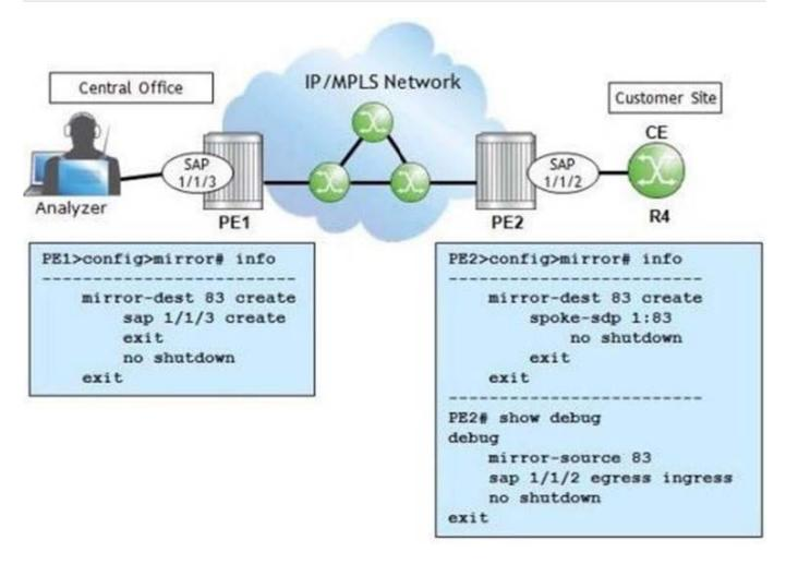
PE1 and PE2 are Nokia 7750 SRs. What needs to be added to PE1\\'s configuration to mirror traffic between PE2 and the customer site?
