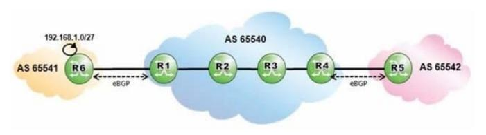
AS 65540 is using MPLS to provide BGP shortcuts for its iBGP routing. Which routers must be configured with the "configure router bgp igp-shortcuts rsvp-te" command?
