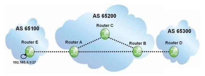
Assuming that none of the routers within AS 65200 is configured with next-hop-self", what will the BGP update for the 192.168.0.1/27 prefix contain when it arrives at router B?
