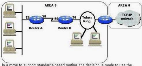
In a move to support standards-based routing, the decision is made to use the OSPF routing protocol throughout the entire network. The areas are shown as in the picture, and the subnets are:
