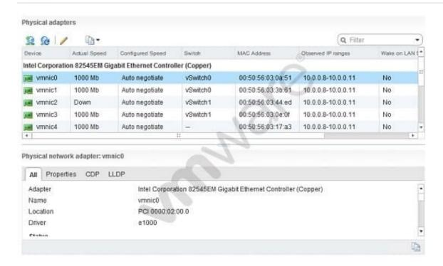
An administrator is configuring an ESXi 6.x host to use multiple NICs to resolve a management network redundancy error. After configuring a second NIC, the server is not able to communicate when the primary connection is taken down. The administrator analyzes the Exhibit shown here.
