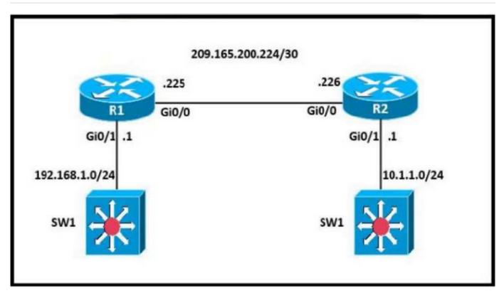
A network engineer is in the process of establishing IP connectivity between two sites. Routers R1 and R2 are partially configured with IP addressing. Both routers have the ability to access devices on their respective LANs.
