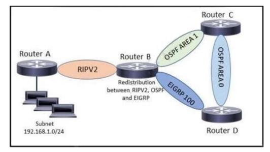
When an administrator executes the show ip route command on router D to view its routing table, which value is displayed for the administrative distance for the route to network 192.168 1.0?
