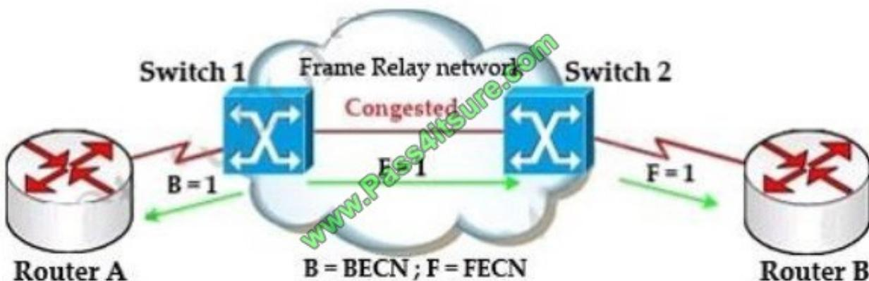
In general, BECN is used on frames traveling away from the congested area to warn source devices that congestion has occurred on that path while FECN is used to alert receiving devices if the frame experiences congestion.
