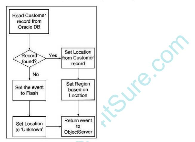
A.Read the Customer record from the Oracle database using the Customer column in the event. If there is no matching record, set the event to Flash, set the Location column to Unknown and return the event to the ObjectServer. If the Customer record is found, set the Location from the Customer record, set the Region column based on the Location and return the event to the ObjectServer.
