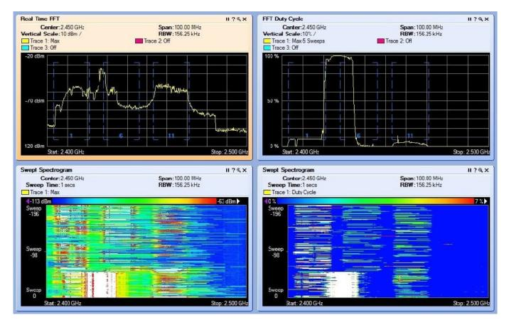
what impact does the video transmitter have on WLAN operations throughout the band?
