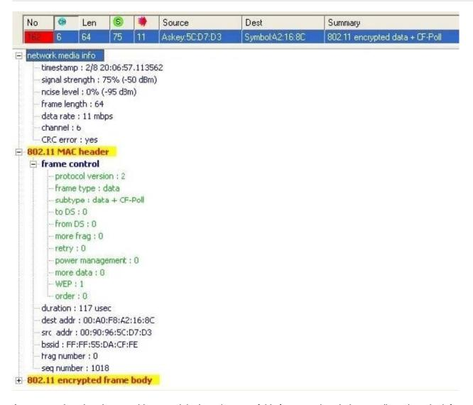
As a protocol analyst, how would you explain the existence of this frame on the wireless medium given the information in the decode?
