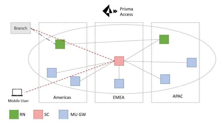
Key: RN -Remote Network SC -Service Connection MU GW -Mobile User Gateway
