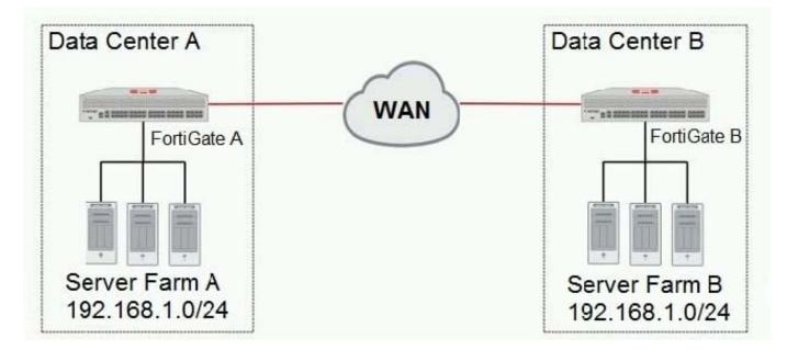
A company has two data centers (DC) connected using a Layer 3 network. Servers in farm A need to connect to servers in farm B as though they were all in the same Layer 2 segment.
