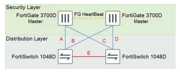
The exhibit shows a full-mesh topology between FortiGate and FortiSwitch devices. To deploy this configuration, two requirements must be met:
