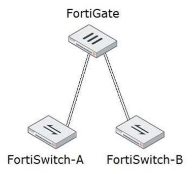
An administrator wants to implement a multi-chassis link aggregation (MCLAG) solution using two FortiSwitch 448D devices and one FortiGate 3700D. As described in the network topology shown in the exhibit, two links are already connected from the FortiGate to each FortiSwitch.
