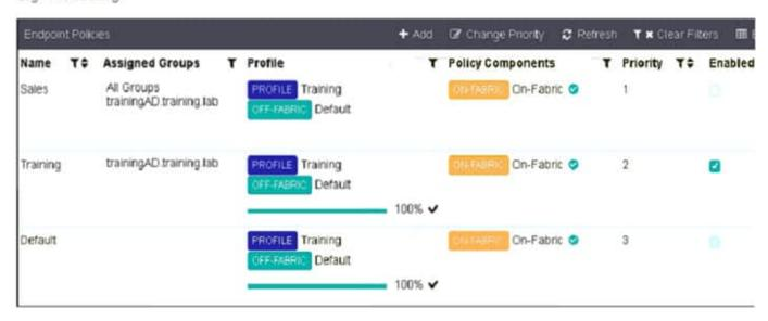
Which shows multiple endpoint policies on FortiClient EMS.
