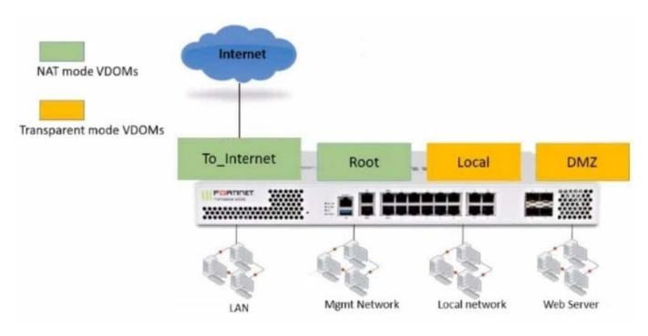
The Root and To\_Internet VDOMs are configured in NAT mode. The DMZ and Local VDOMs are configured in transparent mode.
