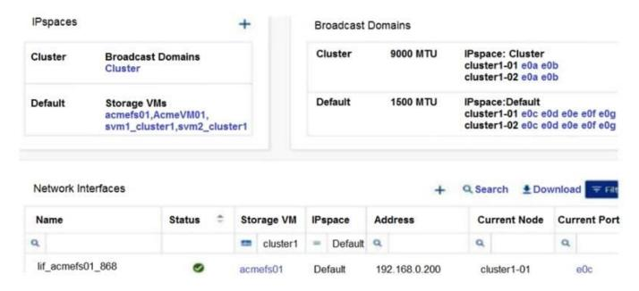
You have an ONTAP 9.8 cluster. After network maintenance, the LIF that is shown in the exhibit is not always on a correct port and is unreachable by users until the LIFs are moved to port eOc or eOd on either storage node. In this scenario, which action should you take to ensure that the LIF only fails over to the correct ports?
