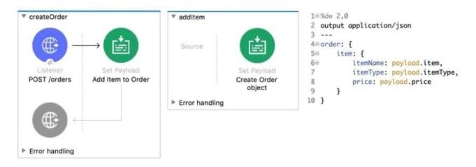
The Set Payload transformer In the additem subflow uses DataWeave to create an order object.
